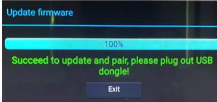
3. Plug out the dongle once the upgrading process is completed. Update all other dongles accordingly.
