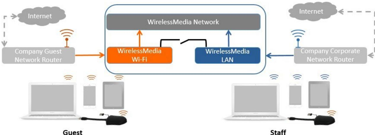
The dongle is connected to the Wi-Fi access Point of the Guest network, which in turn is connected to the internal Wi-Fi access Point of the ALF-WirelessMedia, the dongle can also be configured to connect to the enterprise’s access point. Mobile users stay connected to their current network, have access to their normal corporate environment, as well as Internet access.
