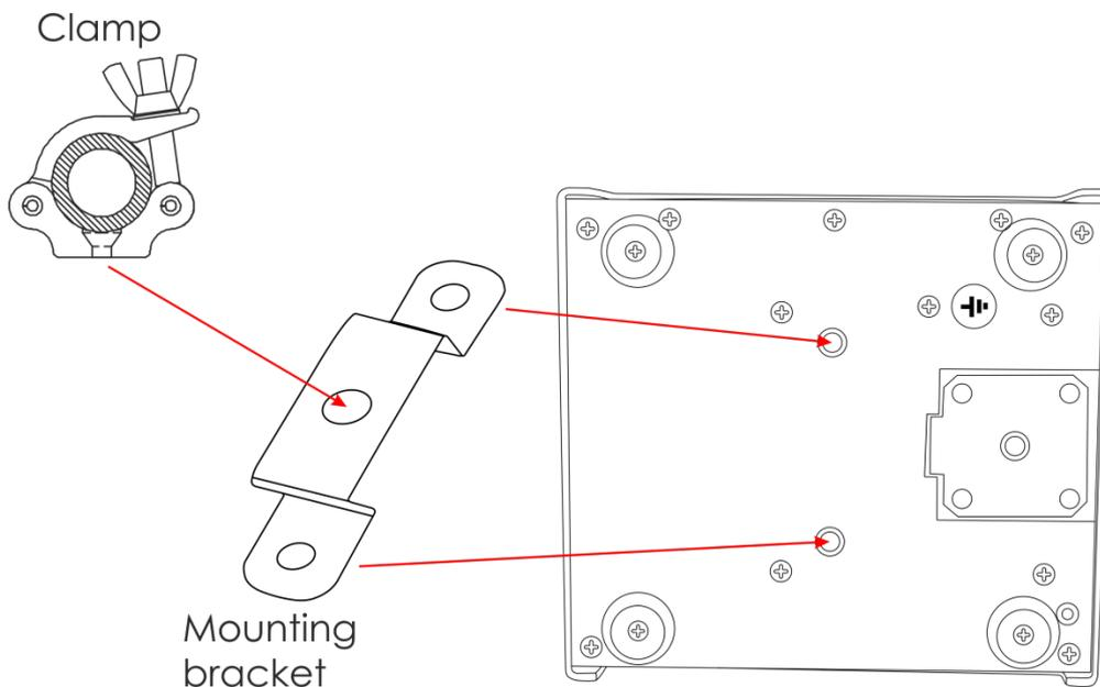
The Kanjo can be placed on a flat stage floor or mounted to any kind of truss with a clamp.
