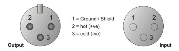
For unbalanced use PIN 1 and PIN 3 have to be bridged
