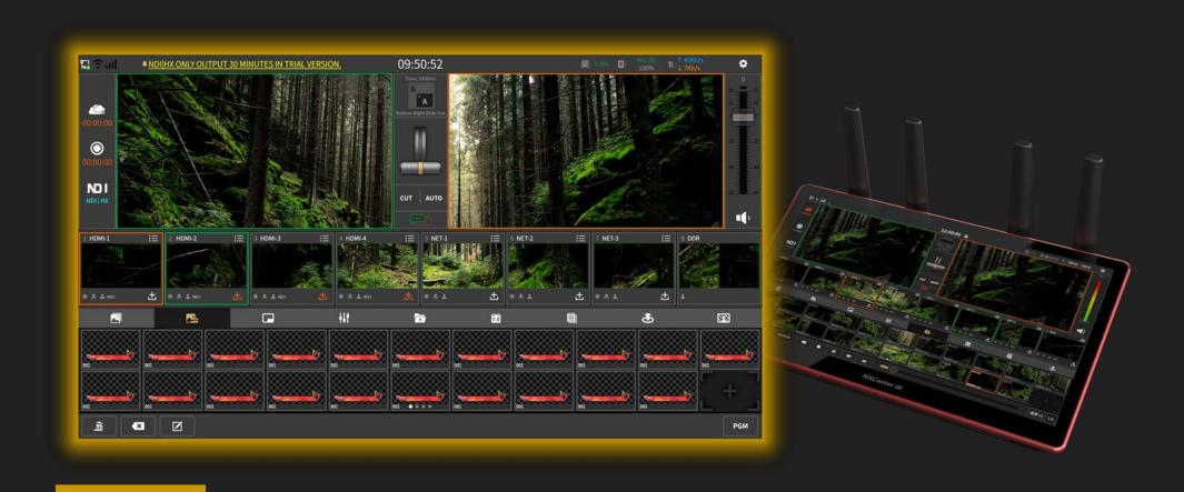
**NSCaster X2** 's CG panel can publish pictures to the PGM channel. It has a built-in large number of pictures but also supports importing external PNG/JPG image formats. Adjusting the position and changing the size of the pictures with up to 20 positions is supported. It is possible to publish imagery on the X2 or remotely with the CG editor software on a PC, making your program production more appealing and comprehensive.
