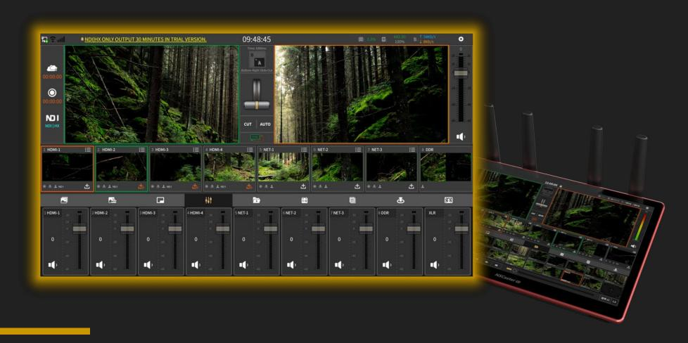
**NSCaster X2** has a built-in software based mixer and supports multiple channel mixing effects. The volume of each input and total output can be controlled accordingly.
