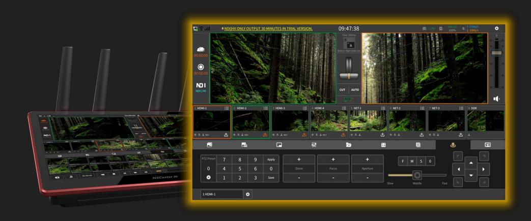
**NSCaster X2** has a built-in PTZ control interface and supports a variety of mainstream PTZ control protocols (visca over IP, onvif, NDI|HX). It can remotely control the camera PTZ, supports zoom, focus and aperture control, supports up, down, left, right, top left, bottom left, top right and bottom right PTZ movement, supports PTZ movement by knob, and quickly locating the target position.
